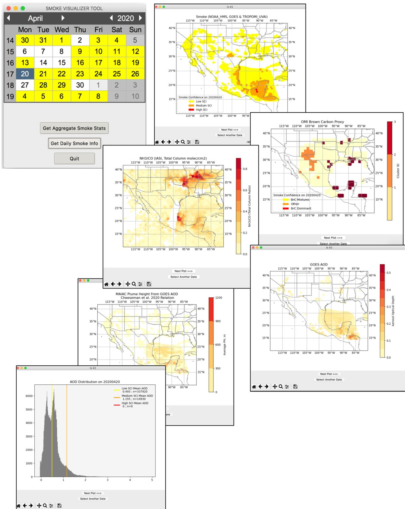
Figure 2. Example GUI Output for Daily Smoke Visualization on April 20, 2020. Additional plots (not shown) include individual smoke pixels for GOES, HMS, and TROPOMI UVAI.
